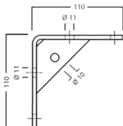
**ANGLE for FIXING of Wire Rope**
