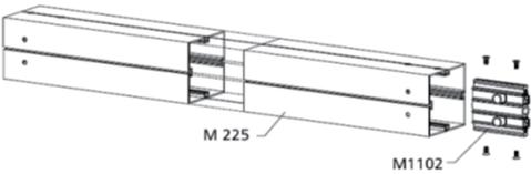
Beam - cut to size w/ Tension locks adaptor M1102 mounted
