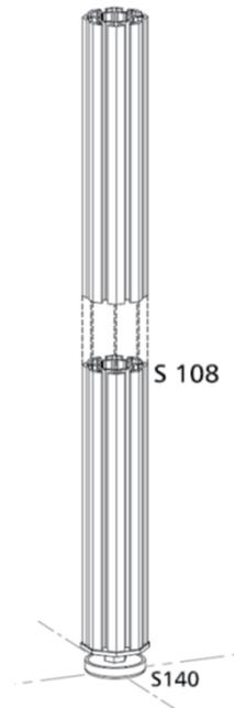
Upright - cut to size with S140 Adjustable foot + M10 thread.
