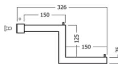
**FRONT SUSPENSION BAR - Staircase Shape**
