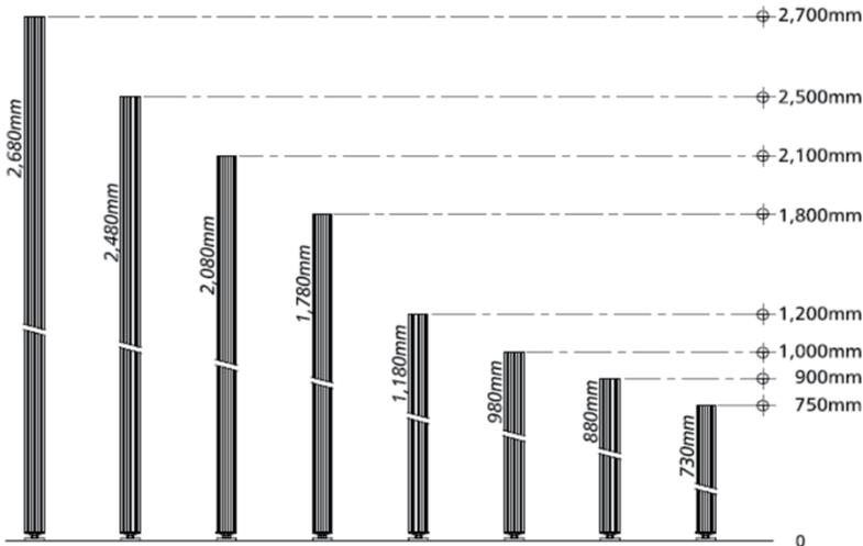
Upright - cut to size with S140 Adjustable foot + M10 thread.
